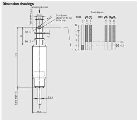
Single hole fixing limit switches must not be used as an end stop.
