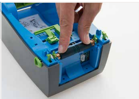
Insert and secure the appropriate roller into the printer.
