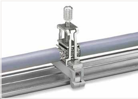
Carrier with grounding foot* (790-113), 45 mm long, busbar 90° to the rail
