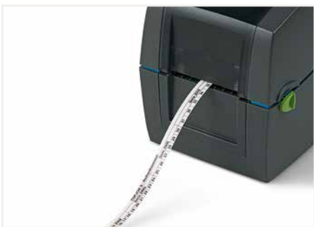
Printing a marking strip (2009-110) via Smart Printer.
