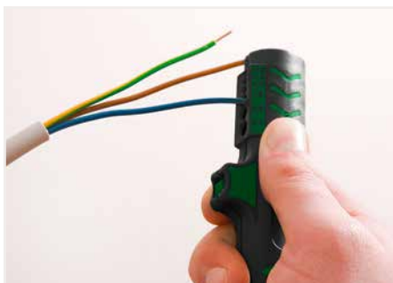
Stripping a conductor insulation.
