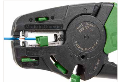
Partially stripping a conductor.
