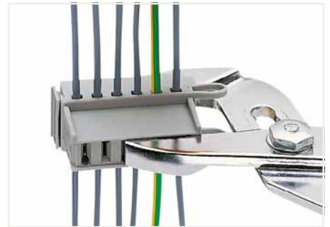
Press into final position using pliers.
