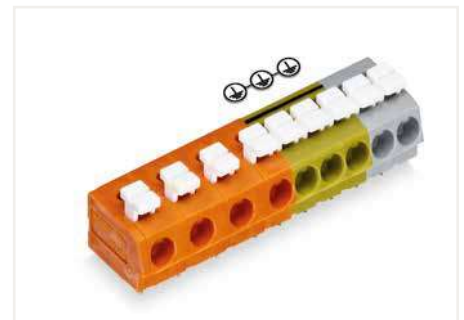
WAGO's 804 Series Terminal Strips provide "internal commoning" to meet requirements that ban routing the ground conductor over the board. This enables custom terminal strips to be commoned and marked at the factory upon request.
