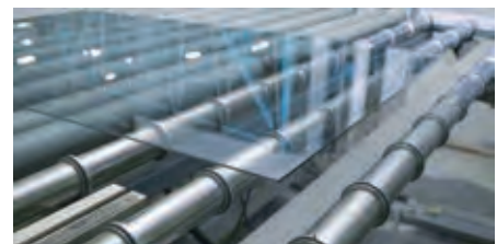
Detection of glass sheet on conveyor
