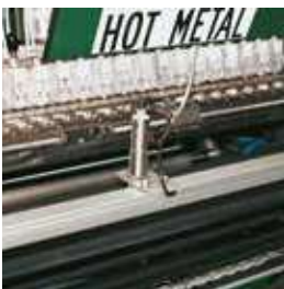
Winding diameter measuring at the laminating machine
