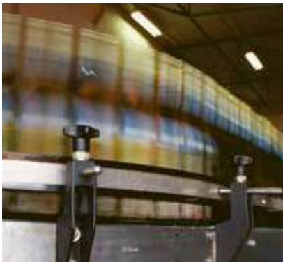
The zws-7, with a 250 Hz switching frequency, is particularly suitable for counting tasks at high machine speeds.
