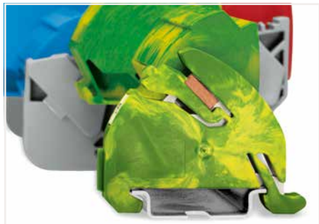
Ground busbar carrier (812-141): Offers a receptacle with locking device for (10 x 3) mm busbar. Contact between the busbar and rail is made automatically by simply snapping the carrier onto the DIN-35 rail. One end of the busbar is mounted onto the ground busbar carrier, the other end is inserted into the middle position of the insulated busbar carrier.
