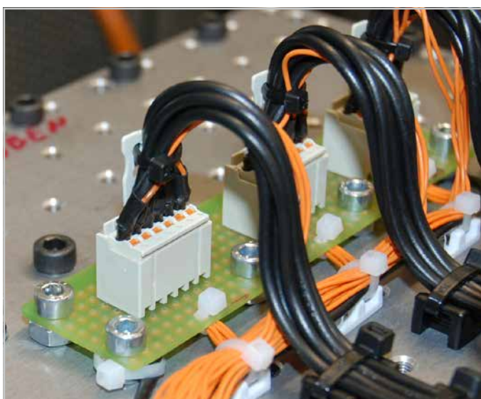
Vibration test performed on a picoMAX® wire-to-board connection (2091 Series)
